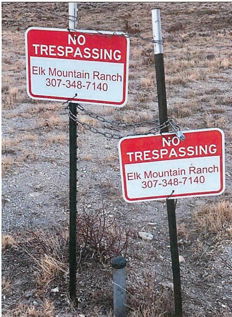
The survey marker (“brass cap”) shown in the photo between the two signs protruding about a foot out of the ground designates the “corner” where Sections 13, 24, 23, and 14 meet. (ECF
